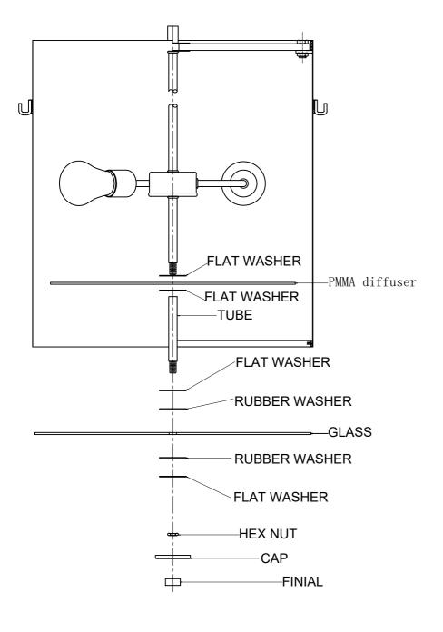
AFTER THE LAMP AND BULB ARE INSTALLED. REMOVE THE GLASS AND PLACE THE FLAT PUT FLAT WASHER THEN DIFFUSER FLAT WASHER USE TUBE LOCK UP WASHER IN THE NIPPLE AND THEN THE RUBBER WASHER. PUT OVER THE GLASS. PUT IT UP INTO THE LAMP BODY. INSERT RUBBER WASHER FLAT WASHER. HOLD GLASS BY HAND AND LOCK WITH HEX NUT. INSERT CAP. LOCK WITH **FINIAL**
